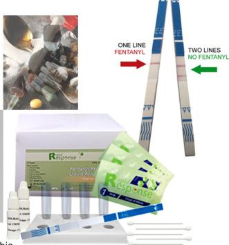
The Fentanyl Forensic Test Kit is a lateral flow Chromatographic Immunoassay for the qualitative detection of Fentanyl in liquid and powder substances at the cut-off concentration of 200 ng/mL.
