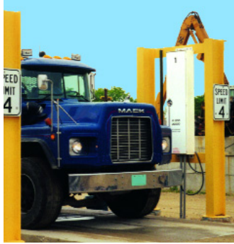
ASM Portal for high-sensitivity truck monitoring – the most reliable 1st line of defense
