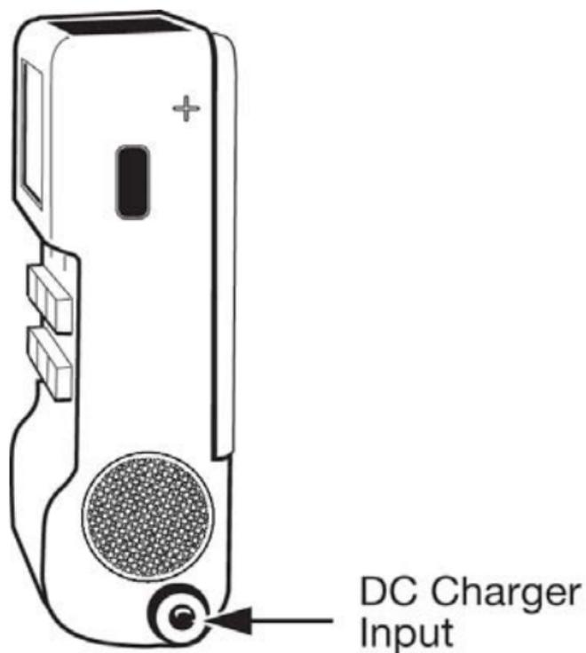
Figure 13 Right Side View of UltraRadiac-Plus
