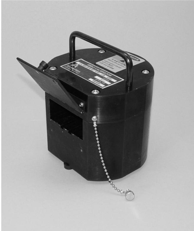
Figure 1 FC2B with Door Lock Screw Removed
