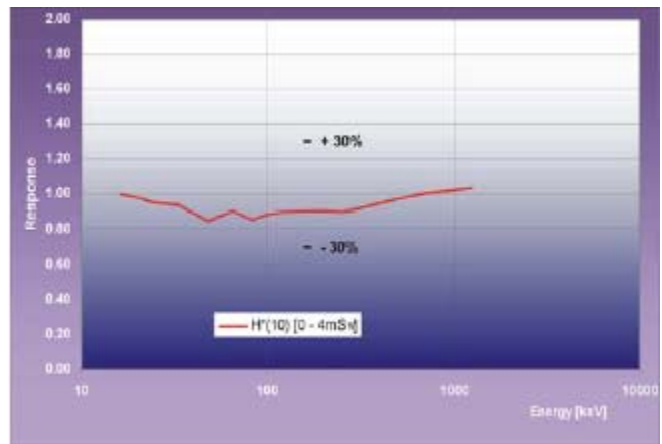
Typical energy response of ambient dose equivalent H^*(10) of more sensitivity element
