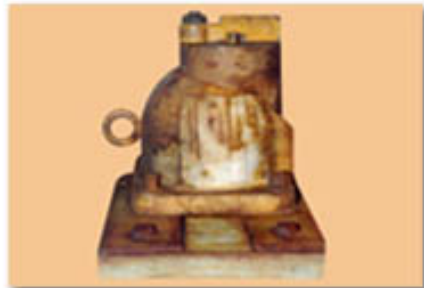
Gauge with oxidation
