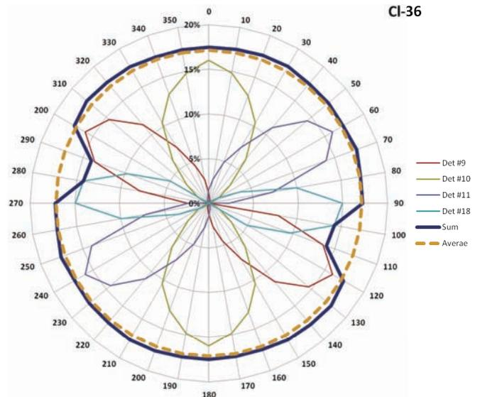
Argos-3/-5PAB Horizontal Scan Efficiency for <sup>36</sup>Cl, IEC 61098 Phantom test 5 cm from center detector.
