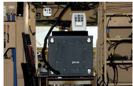
Universal Sampling Port with quick-connect GriffinX-Sorber™ portable air sampler
