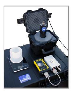
Radioactive material in the sample is detected with a 2x2 sodium iodide scintillation probe using a Marinelli geometry for soil, water, and bulk samples or a 2-inch filter geometry for wipes and air samples. The 500ml beaker is placed in a 1-inch thick lead shield. Depending on the sampling time and the isotope, the detection limit is approximately 60-100 Bq/l and can easily identify concentrations of lodine 131, Cesium 134, and Cesium 137.
