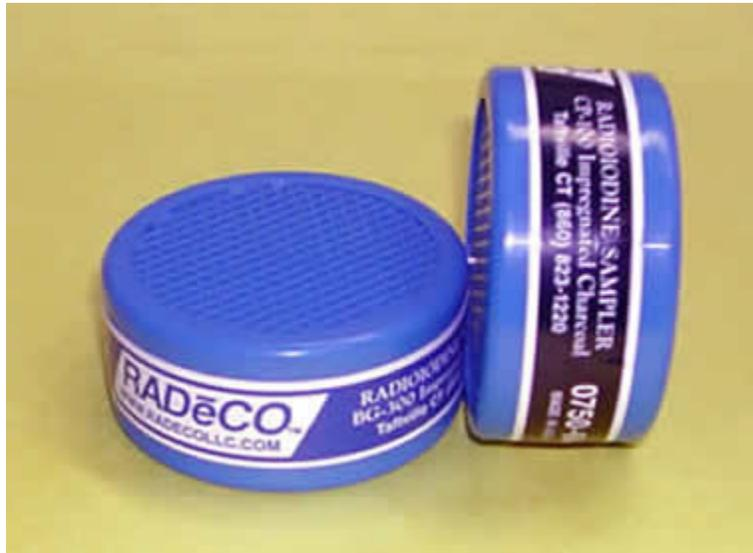
The RADeCO™ Models CP-100 and BG-300 Radioiodine Samplers are special sampling cartridges specifically designed for the evaluation of airborne concentrations of elemental radioiodine, organic radionuclides, and other radioiodine compounds. They are composed of selected 5% TEDA treated charcoal packaged in a plastic case.
