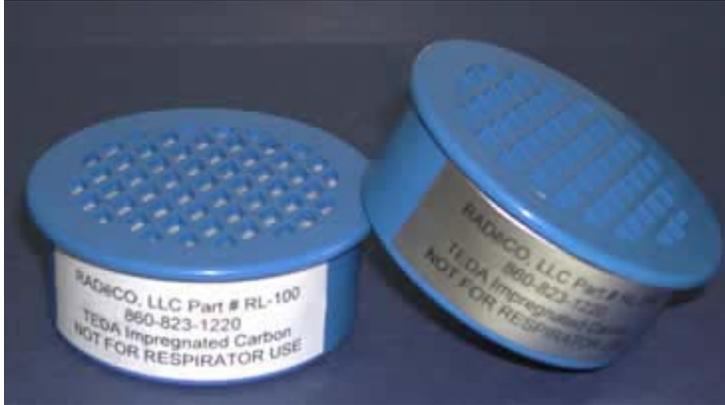
The RADēCO™ Models RL-100 and RL-300 Radioiodine Samplers are special sampling cartridges specifically designed for the evaluation of airborne concentrations of elemental radioiodine, organic radionuclides, and other radioiodine compounds. They are composed of selected 5% TEDA treated charcoal packaged in a plastic case.
