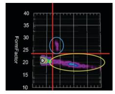
The RadEye SPRD-GN's CLYC and PSD filters provide clear delineation between the gamma radiation of interest (light blue), high energy charged particles typically from cosmic rays (yellow), and neutrons (blue).
