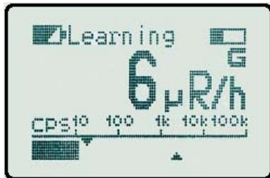
Our screen continuously shows you dose rate. As we are also monitoring count rate you will be alerted by an audible or vibrating alarm if your count rate suddenly increases suggesting you are facing an immediate threat.
