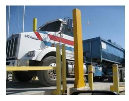
The **RC2W34** Waste Radiation Detection System is a precise and innovative instrument specifically designed to detect radioactive material in a moving vehicle containing waste and scrap. The revolutionary design of the RC2W34 incorporates 20 years of engineering design and proven field application experience.
