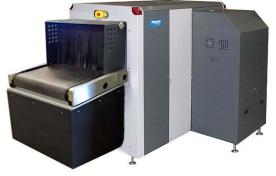
The Rapiscan CM620 is a radiation monitor that automatically and covertly inspects hand-carried articles during X-ray screening at a security checkpoint. The CM620 unit, which contains the radiation detector(s) and electronics, is positioned below the conveyor at the entrance to the X-ray machine. Bags are inspected for radiation as they move on the conveyor over the monitor and into the scanner. A radiation alarm is signaled to the operator by bright lights.
