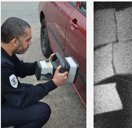
LEFT: MINI Z system scanning passenger door RIGHT: X-ray image of concealed currency
