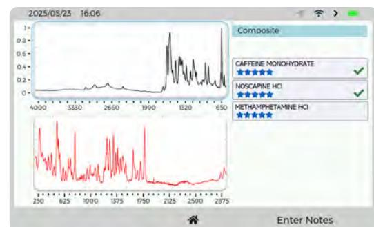
SmartID uses SSP to provide a singular, confidence-based result. Check marks indicate the result was confirmed by both Raman and FTIR.
