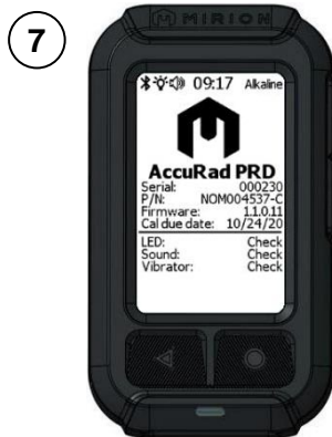
The AccuRad initiates a self-test sequence; wait a few seconds.
