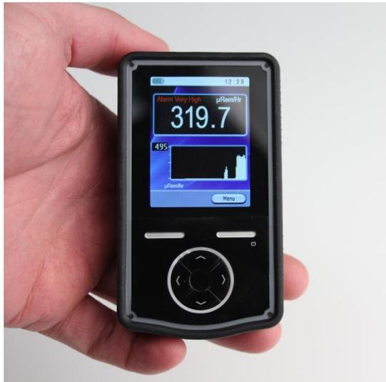
**Figure 1: MiniRad-DX Handheld Radiation Detector**
