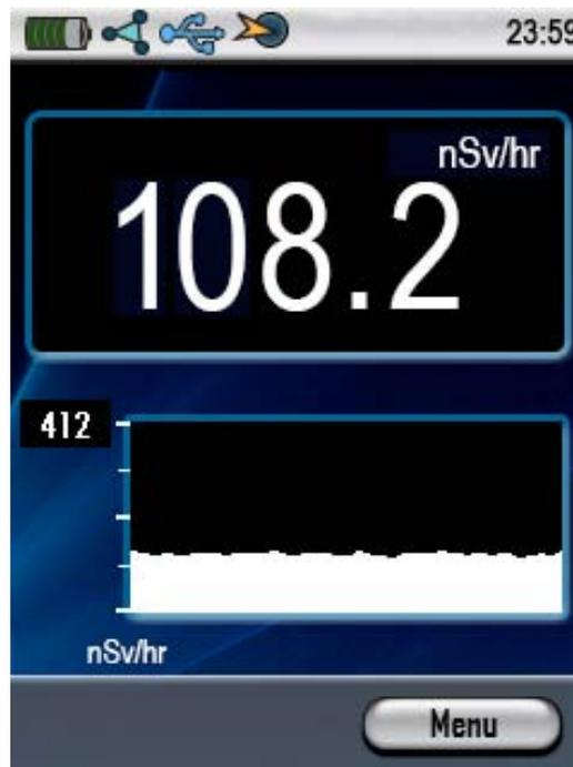
Figure 3: LCD Front Screen: Dose Rate and Graph
