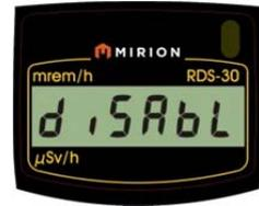
*Note: It is possible to configure the instrument so that the change of the dose rate alarm level is prohibited.*
