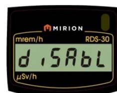
Scroll to check all the valid alarm levels in the instrument. Validating any other value than the diSAbL (with a long press) will enable the multilevel dose rate alarm function.
