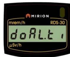
**The dose alarm value used for Time to Dose display is same as the current active alarm level in the multilevel dose alarm mode (see section 2.5.5.2).**
