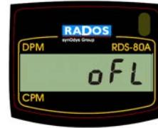
The overflow alarm cannot be reset.
