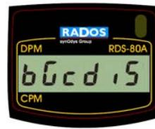
*Note: The background correction will be only performed when the DPM unit is activated. In other words, when the CPM unit is active, no background correction is carried out even if the **bGc on** was selected.*
