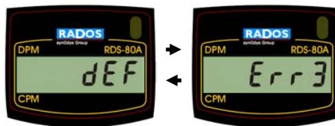
Should an error occur, write down the Error number (**Err+number**) and return the meter for servicing.
