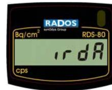
If the communication with the instrument does not commence within 20 seconds, the IrDA link is deactivated and the instrument returns to the contamination measurement.
