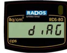
Press the push button shortly to return to the menu or wait 3 seconds to return to the contamination display.
