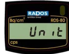
The instrument can be recalibrated to any other isotope using the optional CSW software and calibrated surface source.
