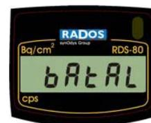
NOTE: The contamination measurement is prevented.
