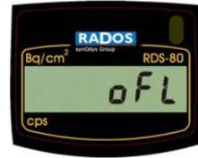
The overflow alarm cannot be reset.
