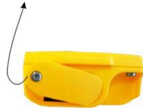
The instrument utilises two IEC LR06/AA-size batteries. The use of alkaline batteries is recommended. The polarity of the batteries is illustrated in the picture on the right. Insert the batteries and lock the battery cap. The instrument is now ready for use. To turn the instrument on, press the push button shortly.
