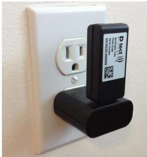
**Figure 11: DX-Link as a Repeater**
