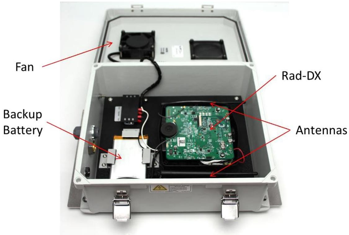
**Figure 5: Inside the NEMA Enclosure**
