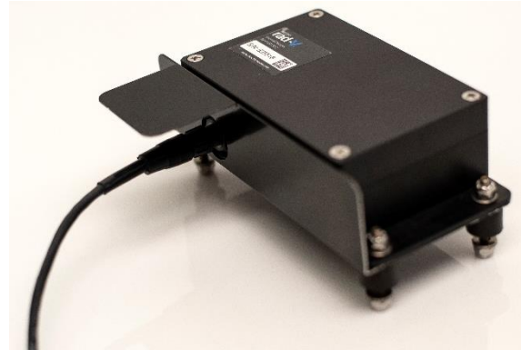
Figure 4: External Detector with Protective Shield
