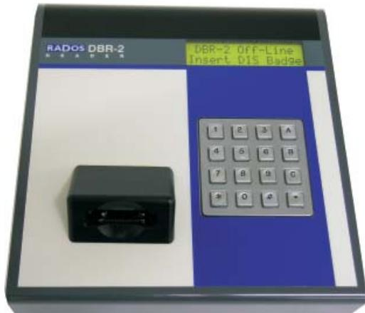
*In the DBR-2 Reader one can instantly read the DIS-1 Dosimeter Badge and transfer the doses to a PC database*
